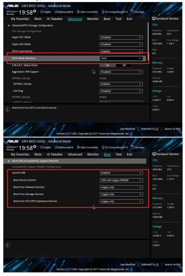
Connect an OptaneMemory device, then enter the OS and select the Optane Installer - ensure that the OptaneMemory device is recognized and appears in the device manager before installation. When using an AHCI OS mode, please select the folder named **Optane**, do not select the **RST** folder.
