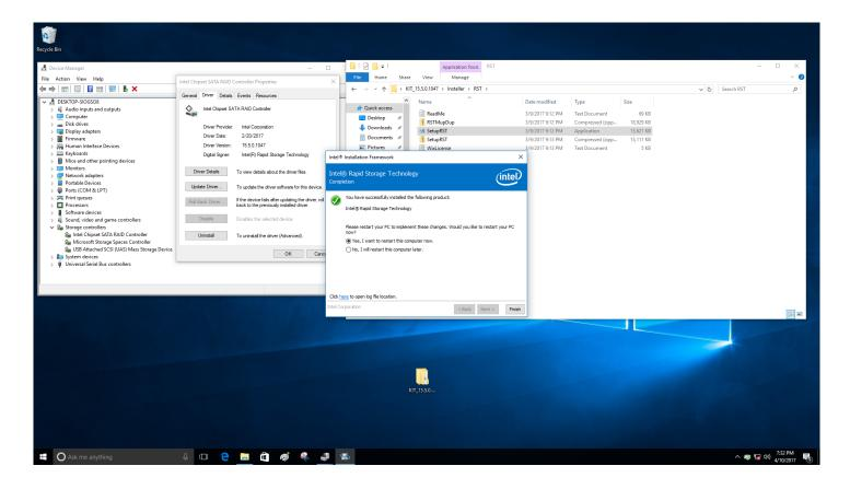
After your computer has restarted, enter the OS and launch the **RST** application, an additional item: **OptaneMemory** should appear. The **Enable** option under the **OptaneMemory** item cannot be selected, this can be activated in the BIOS.
