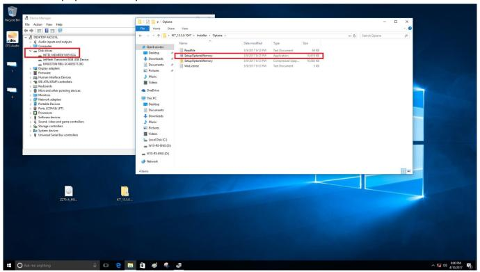
After launching the **SetupOptaneMemory** application, click **Next** and follow the steps shown on the installer. The installer will now prompt you to restart your computer, doing so will transfer **AHCI mode** to **RAID mode**, and **Remapping** options will be set to enabled. If the **CSM** setting is set to default, the **Boot from Storage Devices** option will be set to **UEFI driver first**.
